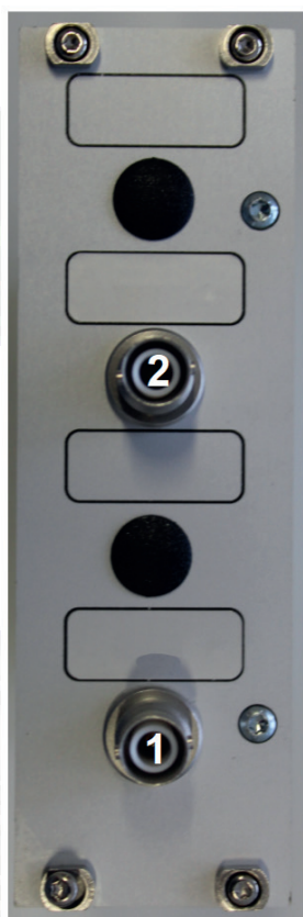
Figure 2: Layout of the 19" HVPS-HC Module R014 (exemplary configuration with a negative output polarity on channel 1 and a positive output polarity on channel 2).
